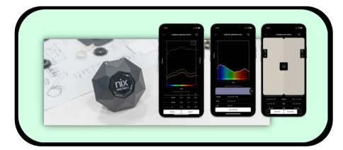
With 1 recorded scan per second, the Nix Spectro 2 has 31 channels across UV, IR and the visible spectrum giving you **unparalleled accuracy and consistent data measurements** time and time again.
