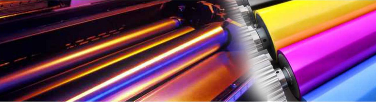
Flexography, also known as Flexographic Printing or 'Flexo', is a method of printing using resilient but flexible raised image printing plates to print on a wide range of flexible substrates including plastic, metallic films, cellophane, paper or cardboard. These presses and the substrate webs they carry can vary in width from narrow to wide web as required by the nature of the work the printer produces.
